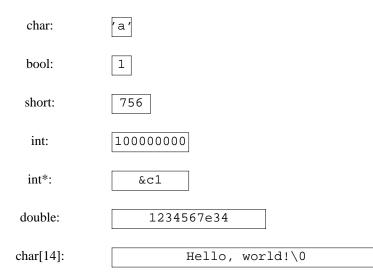
On the same scale (.2 inch to a byte), a megabyte of memory would stretch about three miles (five km) to the right.
