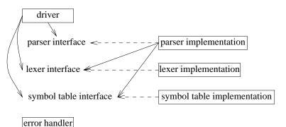
Dashed lines means "implements." I consider this to be the real structure of the program, and our job as programmers is to represent this faithfully in code. That done, the code will be simple, efficient, comprehensible, maintainable, etc., because it will directly reflect our fundamental design.
