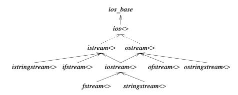
The classes suffixed by <> are templates parameterized on the character type, and their names have a *basic* prefix. A dotted line indicates a virtual base class (§15.2.4).
