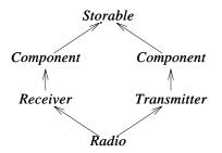
Here, a *Radio* object has two sub-objects of class *Component*. Consequently, a *dynamic\_cast* from *Storable* to *Component* within a *Radio* will be ambiguous and return a *0*. There is simply no way of knowing which *Component* the programmer wanted:
