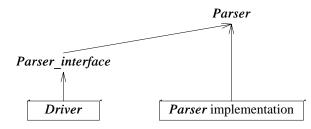
Now the *driver* appears vulnerable to any change in the *Parser* interface from which it was supposed to be insulated. Even this appearance of a dependency is undesirable, so we explicitly restrict *Parser\_interface*'s dependency on *Parser* by having only the relevant part of the implementer interface to parser (that was called *Parser'* earlier) in scope where we define *Parser\_interface*:
