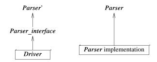
To ensure the consistency of *Parser* and *Parser*', we again rely on the compilation system as a whole, rather than on just the compiler working on a single compilation unit. This solution differs from the one in §8.2.4 only by the extra namespace *Parser\_interface*. If we wanted to, we could give *Parser\_interface* a concrete representation by giving it its own *expr()* function:
