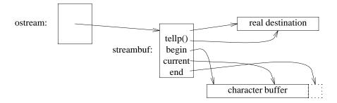
The set of template arguments for an *ostream* and its *streambuf* must be the same and determines the type of character used in the character buffer.
